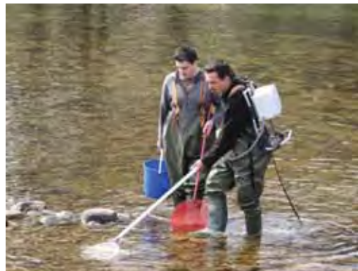
Fish sampling in Nestos/Mesta River using an electrofishing device (from left to right Mr. D. Lachouvaris and Mr. P. Leontarakis) (Photo M. Koutrakis)
